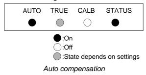
The STATUS LED lights during the automatic distortion compensation functions.
