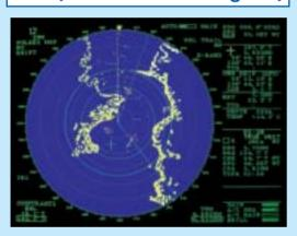
Electronic plotting of 10 targets according to the new IMO and IEC standards. Automatically redraw vectors between manual plots, drops off vectors if not plotted more than 10 min as required by IMO/IEC.
