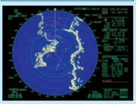
The Auto Plotter ARP-17 automatically tracks up to 20 targets acquired manually or automatically, presents target data, and triggers a collision alarm for the target on a collision course.
